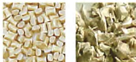
Fig.4 New/ground material
