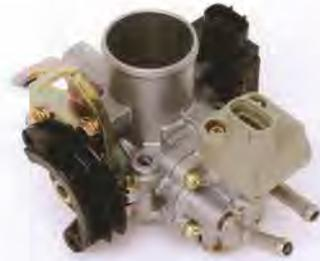
Fig.1 Mechanical throttle body with ISCV
