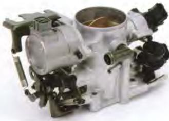
Fig. 3 Mechanical throttle body for UZ engine with non-linear cam device and Traction control valve
