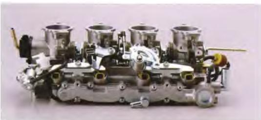
Fig. 4 Independent aspiration throttle for each cylinder
