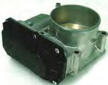
Fig.7 Electric throttle body (4th generation)
