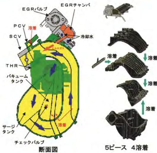
Fig. 3 Composition of Intake Manifold
