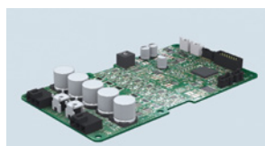
Circuit board required for motor control
